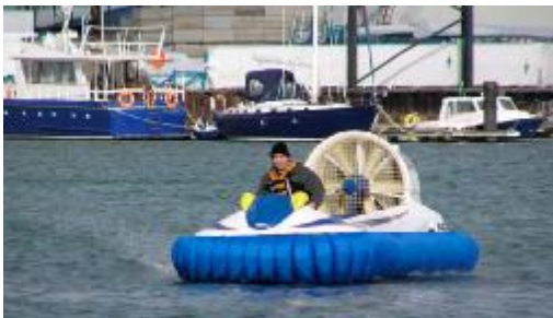
A 2 stroke Rotax –powered HovPod ( www.hovpod.com )
