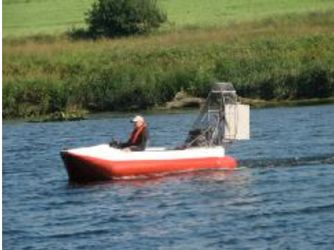
A home-built twin fan SevTec Scout. This craft is capable and extremely quiet. ( http://members.aol.com/sevttec/sev/skmr.html )
