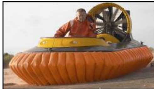
A 2 seat integrated craft from Flying Fish. One engine, one fan, simple and easy to fly. ( www.flyingfishhovercraft.co.uk ) Photo courtesy of www.russpullen.com
