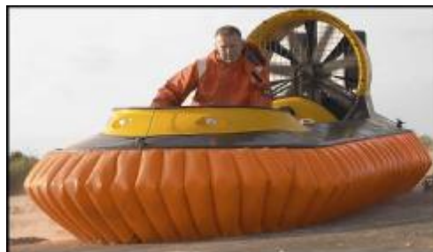
A 2 seat integrated craft from Flying Fish. One engine, one fan, simple and easy to fly.
